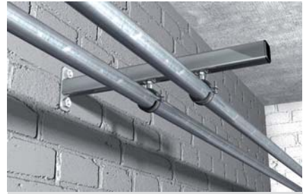
Pipelines on cantilevers
